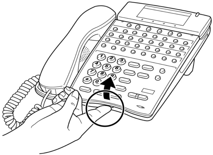
Figure 8-15 Removing the Line Panel
